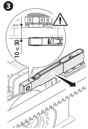
Fasten the support to the rack using the headless screws supplied.
