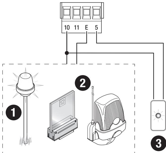
⚠ Maximum contact capacity 10 - 5 24 V AC/DC - 3W
