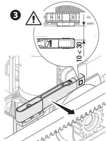
Fasten the support to the rack using the headless screws supplied.
