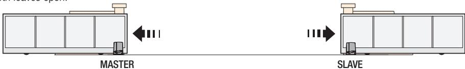
PARTIAL OPENING command. Only the leaf on the MASTER operator opens until it reaches the partially open point programmed in [Set up gate travel].
