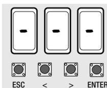
4. Press and hold the button labelled with the arrow < and check whether the operator opens.
