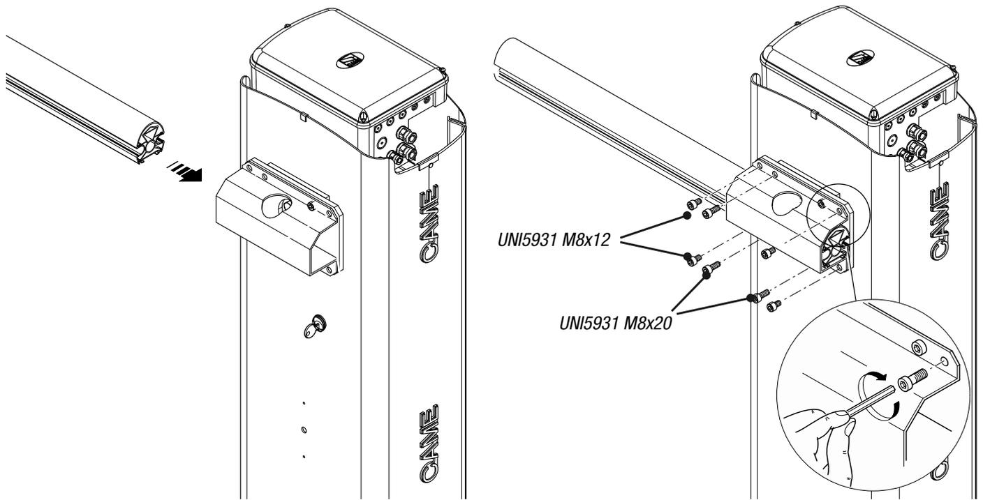
Cut the groove covers to the required length and insert them in the boom conduits on both sides **1** **2**.
