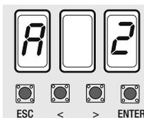
2. Select 1 to activate the test. Press ENTER to confirm...
