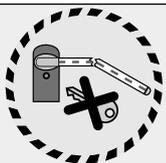
⚠ **Caution!** The release operation is potentially hazardous for users when the taut springs no longer guarantee correct balance. This may occur if the boom is badly fastened, ripped out or broken during an accident, for example. This could lead to a sudden rotation of the boom attachment and/or of the boom itself.
