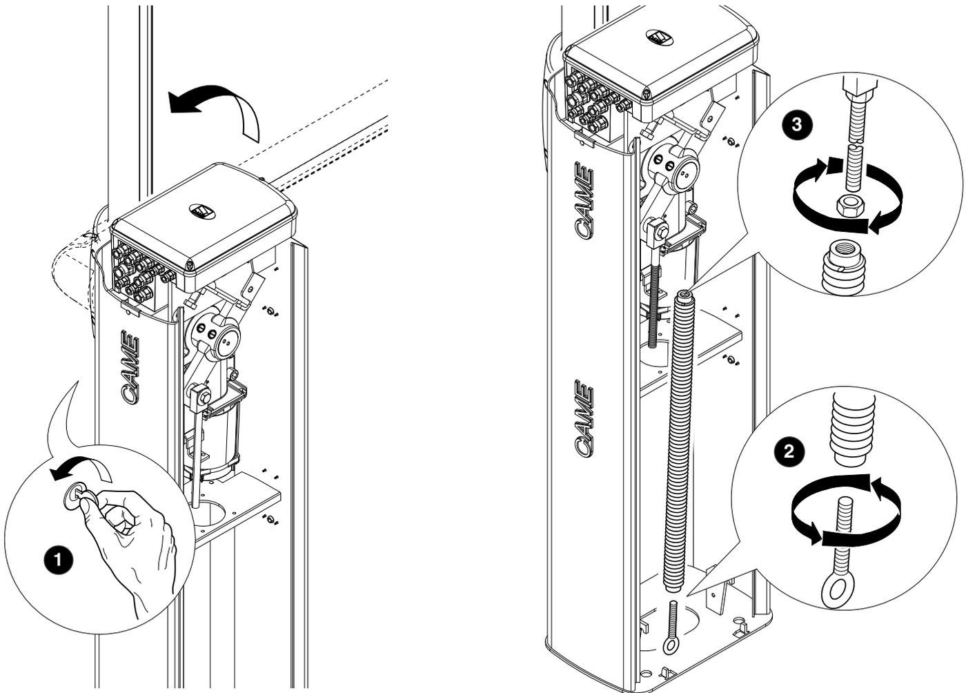
Hook the eyelet rod onto the anchoring bracket **4**.
