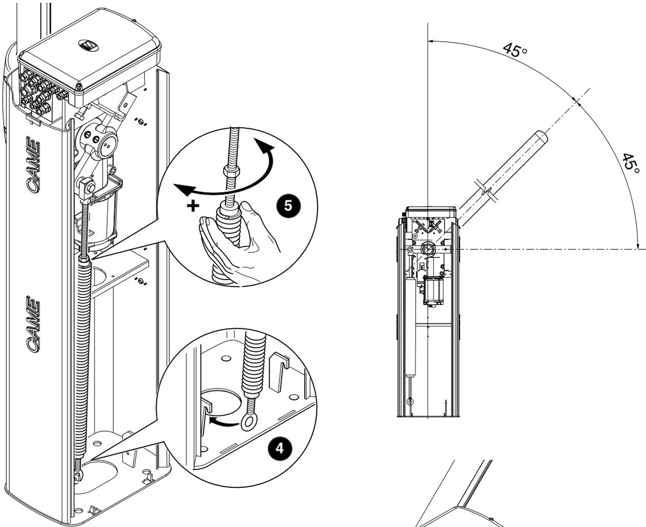
Fix the counter nut and lock the gearmotor again.
