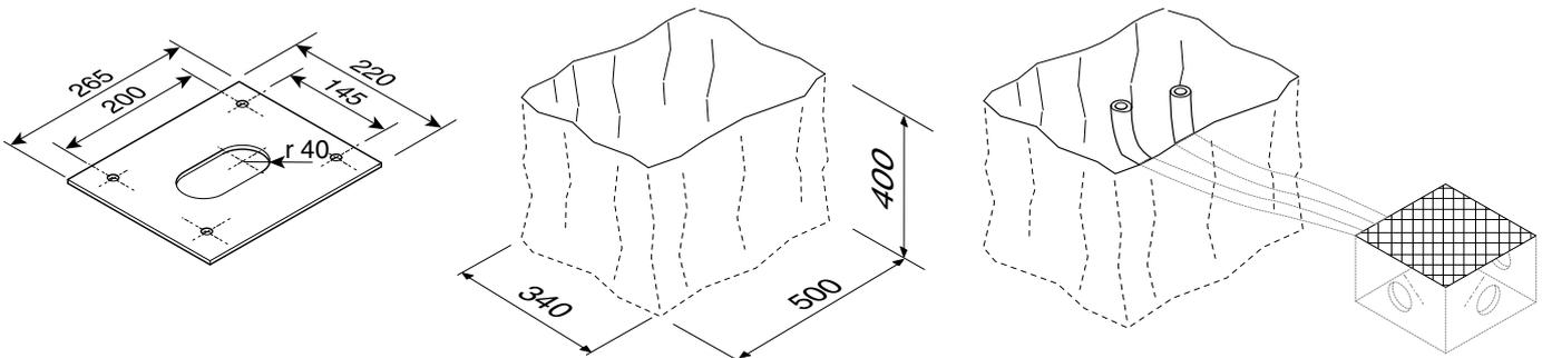
Prepare a foundation frame that is larger than the anchoring plate and sink it into the dug hole.
