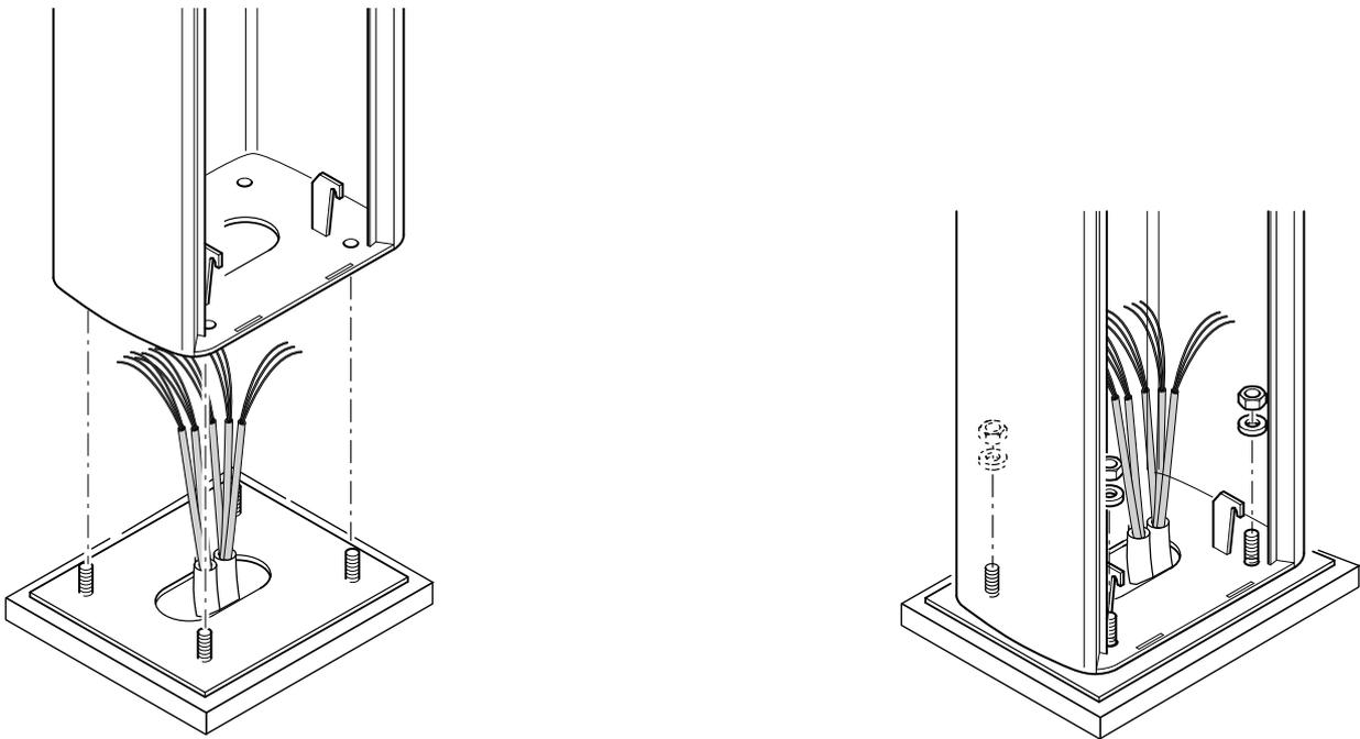
Attach the intermediate plate and boom-attachment cover to the attachment plate with a screw. Leave the screw loose to make it easier to insert the boom.
