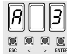
2. Select 1 and press ENTER to confirm the automatic travel calibration.
