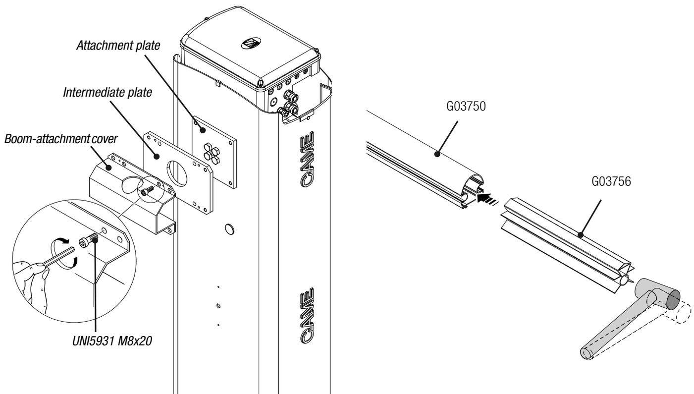
Fit the boom into the attachment cover and fasten it using the screws.
