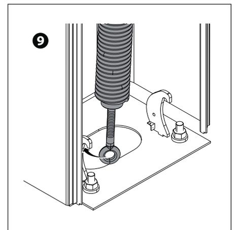
Lubricate the spring when it is fully extended.
