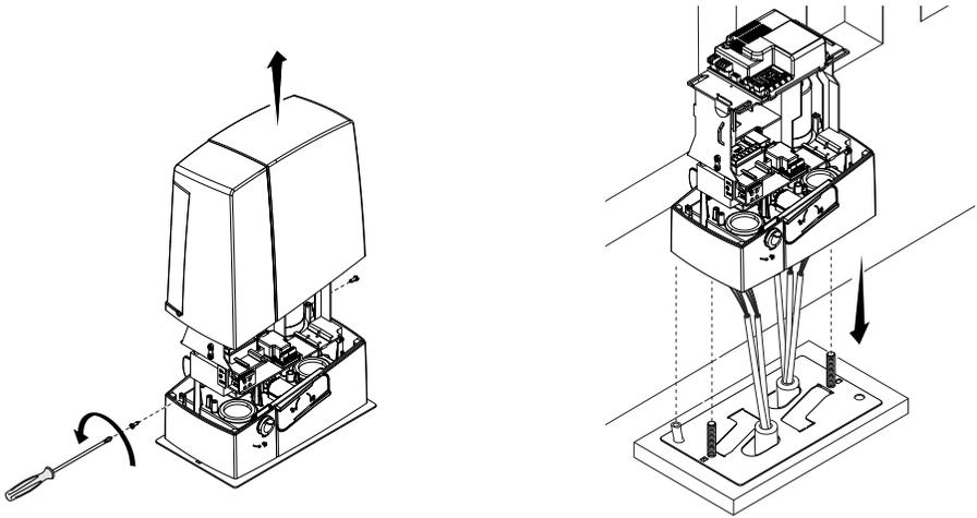
Perforate the cable gland, pass the cables through and fit it into its corresponding housing.
