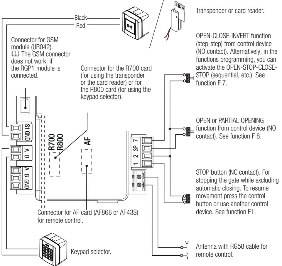
To be able to snap in the cards into the dedicated connectors, remove the card cover.
