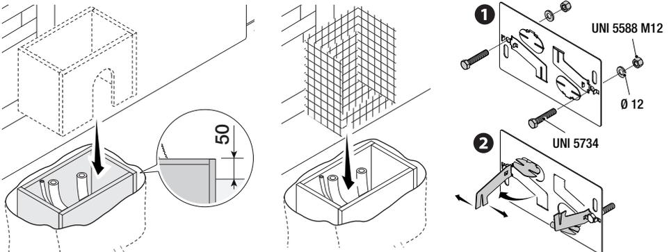
If the rack is already there, place the anchoring plate, being careful to respect the measurements shown in the drawing.
