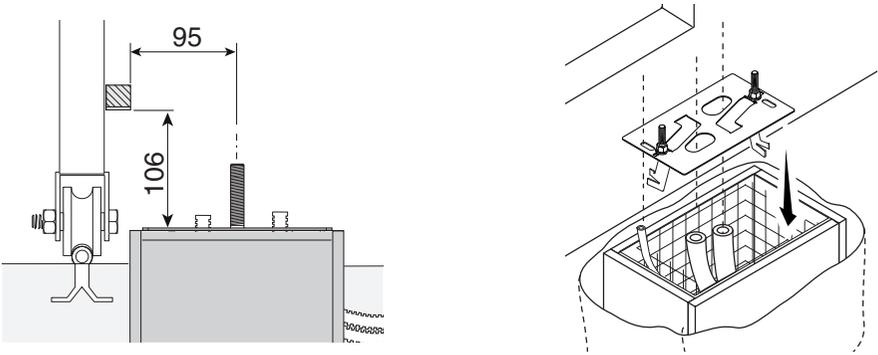
Fill the foundation frame with concrete. The plate must be perfectly level with the bolts which are entirely above surface.
