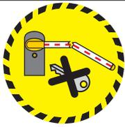
**⚠ WARNING!** The release action may result in danger for the user, when, for whatever reason - the arm is improperly fixed to the pin during mounting, the arm is broken or cracked during an accident, etc.- the tension springs no longer provide balance! **This may result in sudden rotating movements of arm attachment and/or of the arm itself.**
