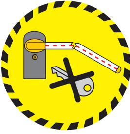
**⚠ WARNING!** The release procedure may constitute a hazard for the user when, for whatever reason – the bar is fixed improperly to the housing during assembly, or the bar is cracked or broken in an accident, and so on – the tension springs no longer provide balance! These can thus cause a brusque rotation of the bar attachment and/or of the bar itself.
