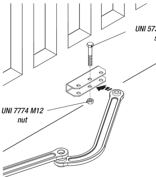
Release the gearmotor and secure the driven arm to the gate-attachment bracket using the nut and bolt.
