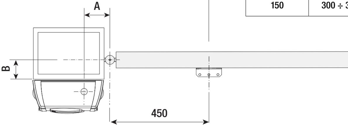
Mark the fixing points for both the pillar and gate brackets, respecting dimensions indicated in the drawing.
