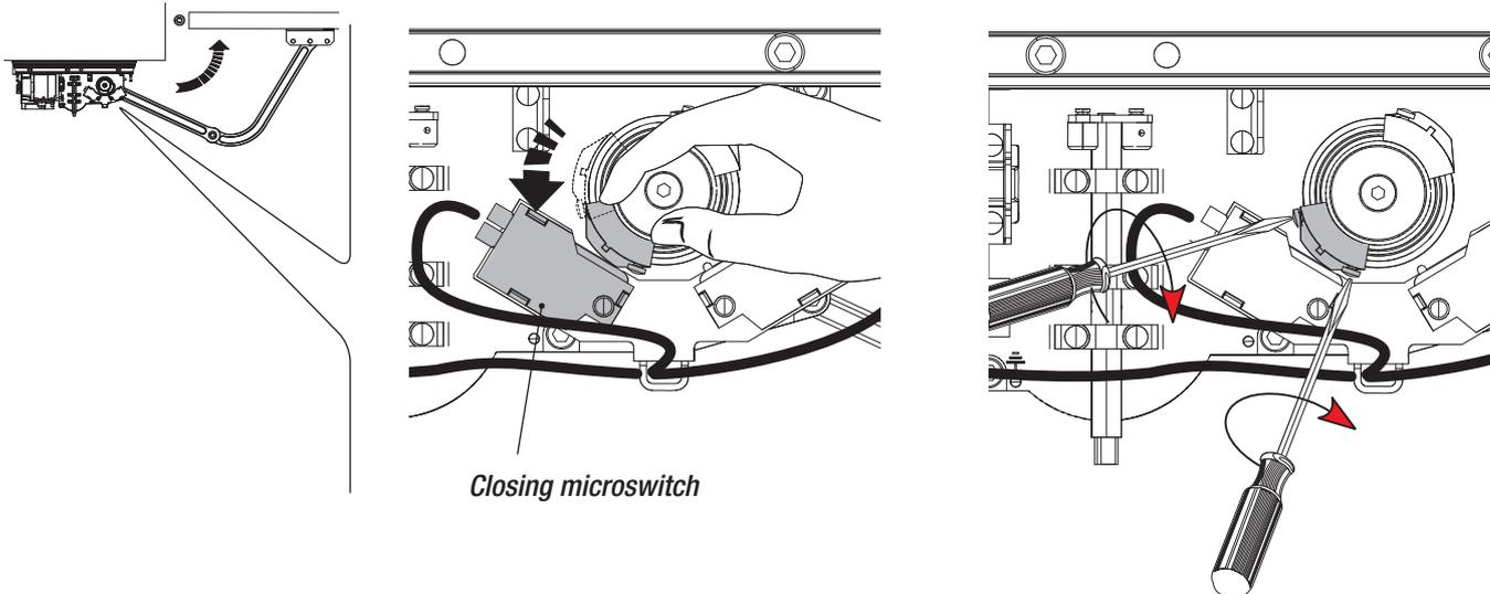
Fully open the gate-leaf of the left gearmotor and rotate the cam counter-clockwise until the opening microswitch inserts. Fix the cam with the screws.
