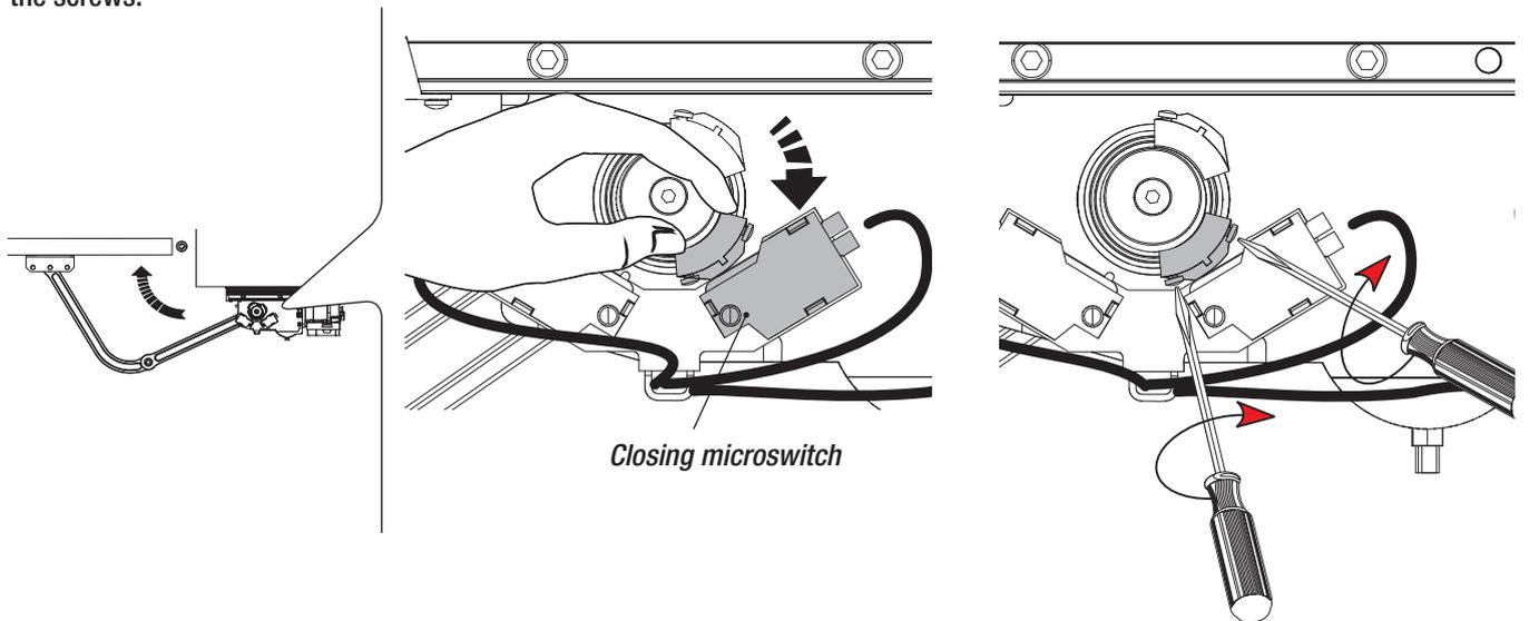
Fully open the gate-leaf and rotate the other cam counter-clockwise until the opening microswitch inserts. Fix the cam with the screws.
