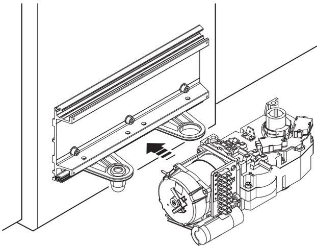
Insert the gearmotor on the plate.
