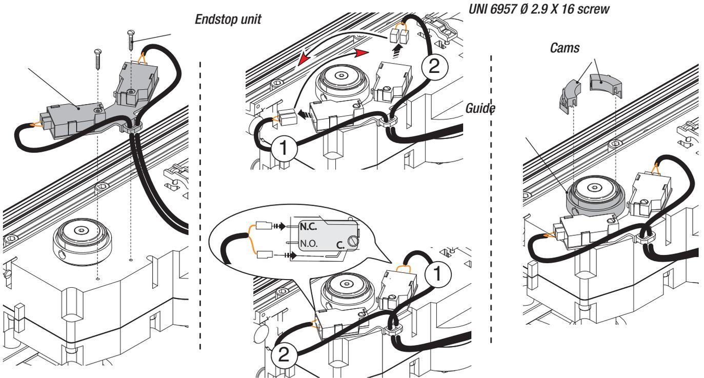
Fully close the gate-leaf of the left gearmotor and rotate the cam clockwise until the closing microswitch inserts. Fix the cam with the screws.
