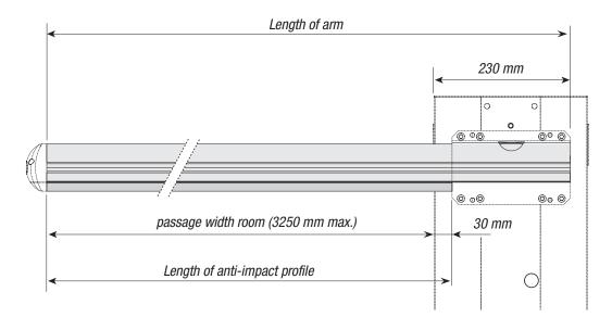
Calculate the am length and that of the anti-impact profile by using as reference the passage width room.If necessary, cut any extra parts.
