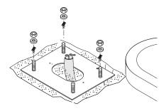
Warning: the barrier must be mounted by at least two persons. Use proper hoisting equipment when transporting the barrier. During mounting phase, the barrier may be unstable. Do rest against barrier until fully mounted, to avoid any tumbling over.
