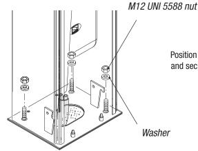
Position the cabinet to the anchoring base and secure it using the washers and nuts.
