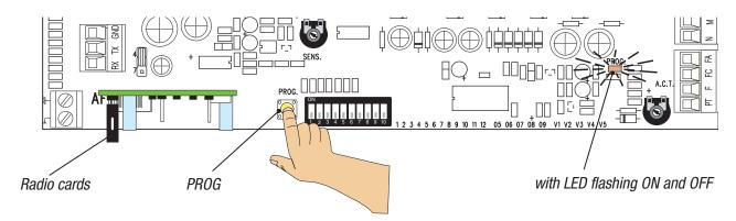
Press the button on the transmitter to be memorised. The LED will stay ON to confirm memorisation is OK.
