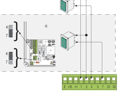
Immediate closing (N.C.) Contact Immediately closes the barrier after vehicle has passed within the oeprating range of the safety devices. if unused, set Dip switch 8 to ON.
