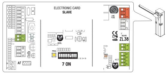
At the end, connect the two cards together using the terminals **RX-TX-GND**.
