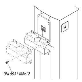
Position the arm-attachment cap against the transmission shaft plate with just one screw and leave this loose.
