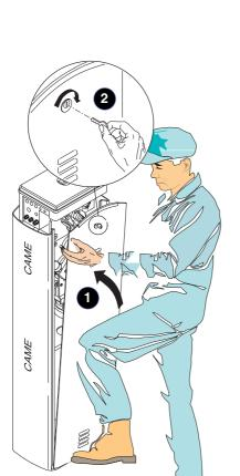
5) Insert the inspection hatch and close it.
