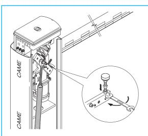
3) After bar opening and closing adjustment, tighten the locking nuts under the dampers.
