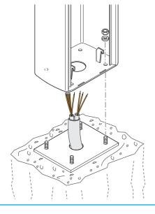
4) Remove the nuts and washers from the threaded screws, position the cabinet on the base in correspondence with the 4 threaded screws and secure with the nuts and washers.
