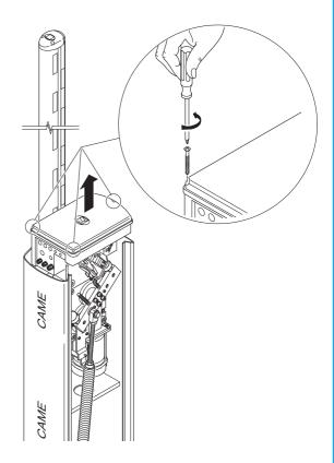
2) Insert the board in the container and fasten it with the screws provided; carry out all the electrical connections (see the dedicated technical documentation enclosed with the board).
