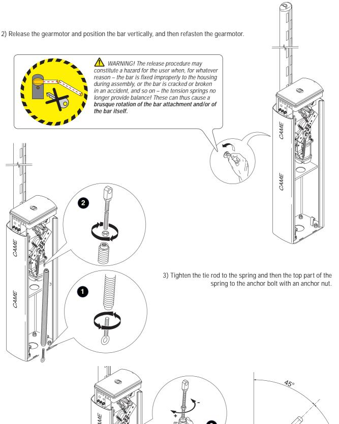
4) Hook the tie rod to the anchoring bracket, release the gearmotor and manually turn the spring to increase or decrease traction until the bar rests at 45°.
