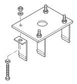
2) Assemble the four anchoring clamps at the base.
