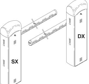
2) The barrier is designed to be installed on the left of the gateway as seen from inside.
