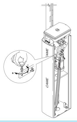
2) The procedure is similar for the bar's opening position. Adjust the closure damper screw until a position parallel to the road surface is reached.
